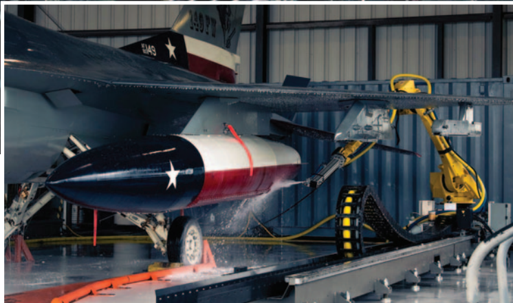
While it looks similar to a commercial de-icing setup, the jet-washing robot is customized to clean the F-16, so it can get to even hard-to-reach areas. (U.S. Air Force image by Senior Airman Ryan Mancuso.)
