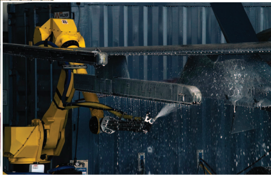
The jet-washing robot is effectively hosing down one of the F-16's pylons. (U.S. Air Force image by Senior Airman Ryan Mancuso.)
